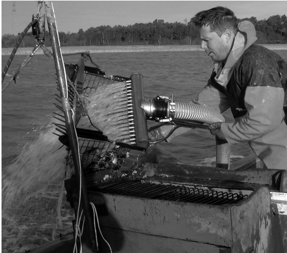
Figure 3 A pump-scoop used in the Poole clam fishery.
