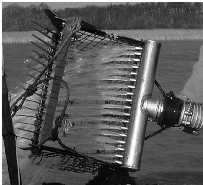
Figure 3 A Poole Harbour clam pump-scoop. Note how the water jets enter the front of the scoop and wash the sediment out of the basket.
